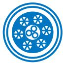
CSP sheath. Positive trackfeeder cables commonly used include 1x1000mm<sup>2</sup> (aluminium), 1x630mm<sup>2</sup> (copper) and 1x500 mm<sup>2</sup>(aluminium). Negative trackfeeder cables commonly used include 1x800mm<sup>2</sup> (aluminium), 1x500mm<sup>2</sup> (copper), 1x240mm<sup>2</sup> (aluminium), 1x161mm<sup>2</sup> (copper) & 1x150mm<sup>2</sup> (aluminium). The applicable standard is NR/PS/ELP/21101. BS6360 and BS6899 for UK Network rail and NF-F5525 for France RATP.
